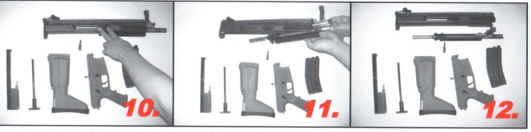
10. 使用梅花扳手轉開左右側槍管結合螺絲 Remove the two barrel fixed (star) screw on both side middle of upper receiver. 11. 向前向上分離槍管總成 Push forward the barrel sets forward 4.5 cm and pull up to take out the barrel sets. 12. 大部分分解完成(反向即可組裝恢復) Complete.(Please reverse step to complete installation)
