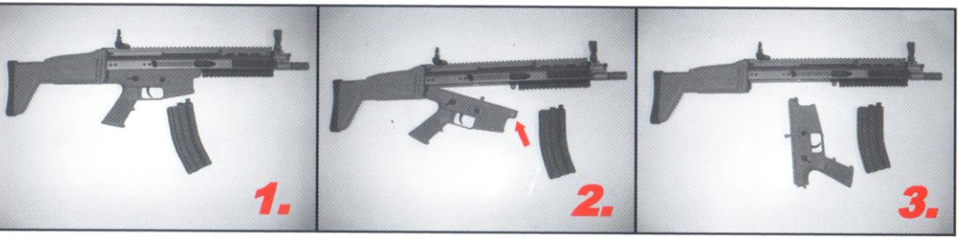
1. 卸除彈匣。拉拉柄確認無殘留BB彈在槍腔內，關保險 Remove the magazine. Pull the charging handle to lock the hammer and turn the fire selector to SAFE(S) position. 2. 由左側推出下槍身結合銷 Pull the charging handle back around 2cm and push the lower receiver locking pin out. 3. 向下向前拉出下槍身 Pull out the lower receiver from front.
