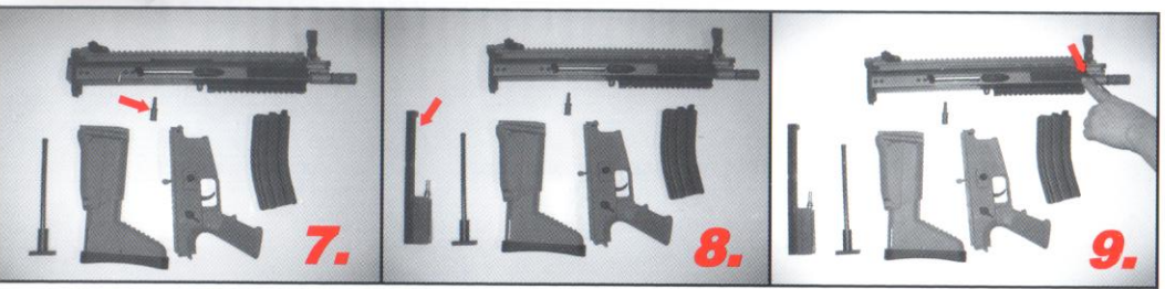
7. 取出拉柄並倒出槍機 Take the charging handle out. 8. 取出槍機 Remove the bolt carrier module. 9. 使用梅花扳手轉開左右側前結合螺絲 Use the star key tools(Gas regulator) to remove the barrel fixed (star) screw on front of both side rail.
